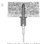
Attach the M8 or M10 Stud end fixing.
