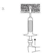
Use a hammer to drive in the setting punch to expand the anchor
