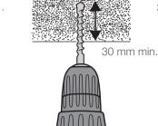
Drill concrete (Use wire brush to ensure the hole is clear)
