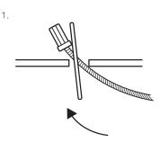
Push the toggle plate so that it is parallel to the rope
