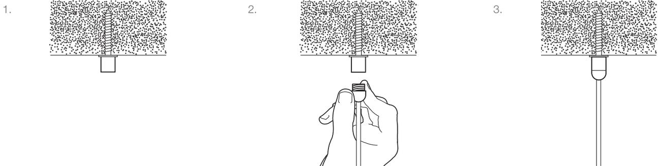
Fix using M6 or  $\varnothing$  4.5 mm c/sunk screw
